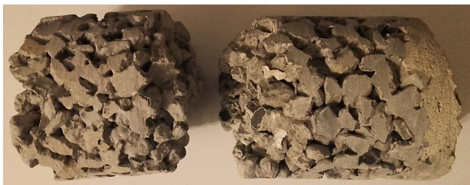
Fig. 2. Sample of the NFC wall formed by 280mm NFC and 15mm thick external render
