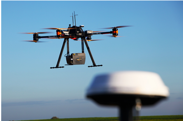
Figure 2: Commercial Drone with Aerial Mounted LIDAR [source: Cargyrak, Wikimedia Commons, accessed 4/29/2018]
