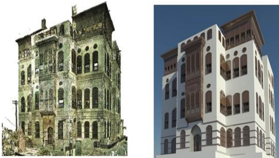
Fig.4. On the left side is a house of Nassif, a product with a laser scanner, and on the right side is a building information model for the historic house of Nassif in Jeddah, Saudi Arabia JHBIM. [4]
