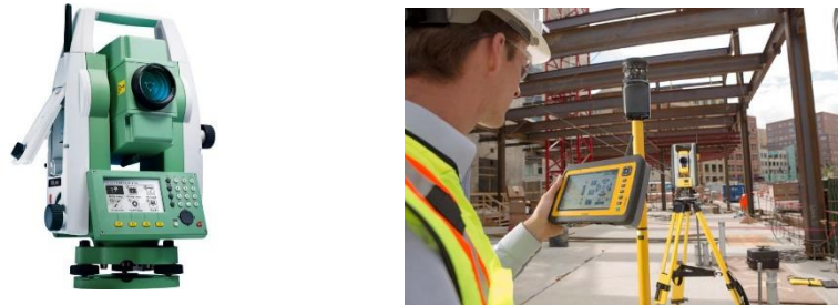
Figure 1: (a) Two-man Total Station (b) Robotic Total Station
