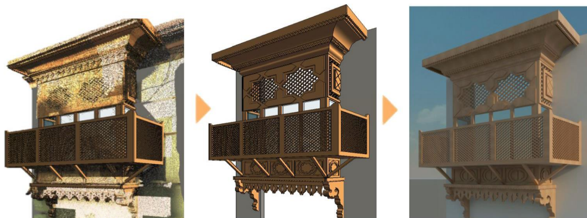
Fig.2. Creation and visualization of a 3D model based on a point cloud. Source (Jeddah Historical Building Information Modelling "JHBIM" – Object Library)
